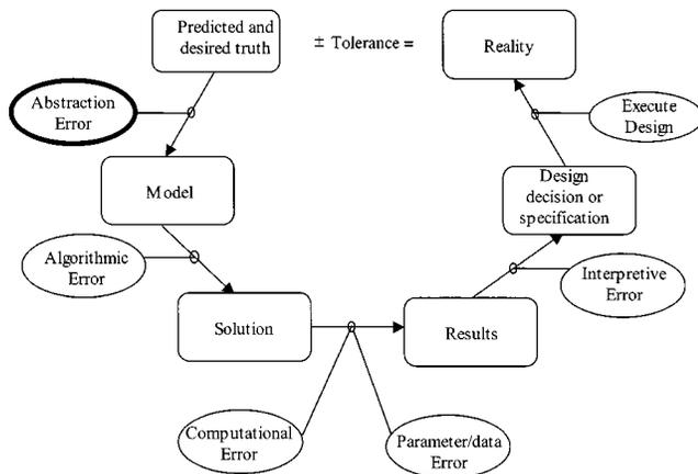
Fig. 2 Schematic showing sources of error in engineering design models
