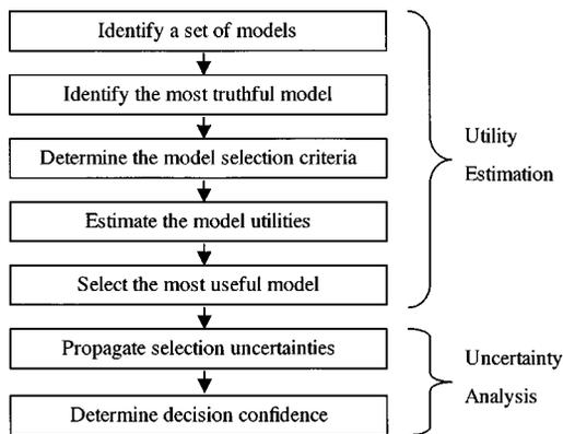
**Fig. 4 Diagram showing the steps of the Model Sufficiency Estimation Technique**
