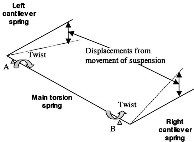
Fig. 6 Schematic showing the operation of the sway bar system
