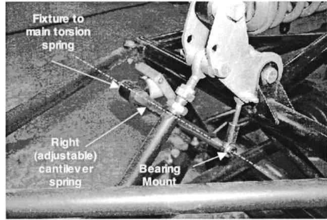
Fig. 7 Close-up view of the cantilever spring in flat position
