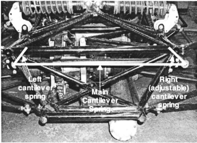
Fig. 5 View of the sway bar system (from the rear of the car)
