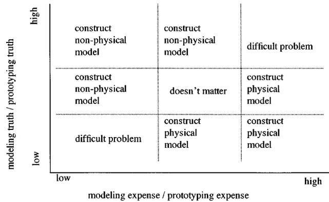
Fig. 3 Tool used for model selection guidance (adapted from [3])
