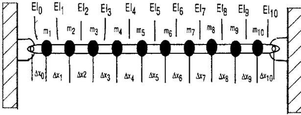
Fig. 11 Lumped model for a pinned-pinned beam
