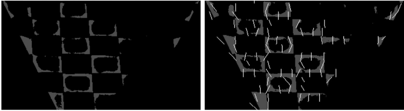
Fig. 10 Left: image of the checkerboard tiled floor after the adaptive threshold is applied; right: image of the checkerboard tiled floor after least-squares regression is applied.
