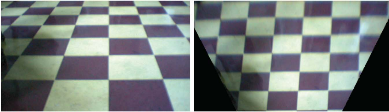
Fig. 9 Left: original image of the 1- × 1-ft (30.48-cm) checkerboard tiled floor with distortion; right: image of the checkerboard tiled floor with the perspective corrected. (Color online only.)
