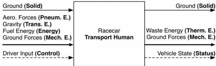
Figure 6 shows a conceptual level functional model. Such a functional model is consistent with one created during a conceptual design project in which there are few constraints or assumptions about the use of the vehicle. As the goal here is to create a quantitative vehicle dynamics model from a functional model, the functional model development extends with this specific focus.
