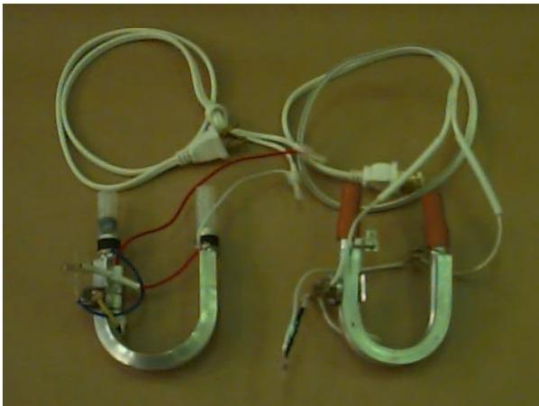
**Fig. 3.** The convert electricity to thermal energy module for both tea brewers.
