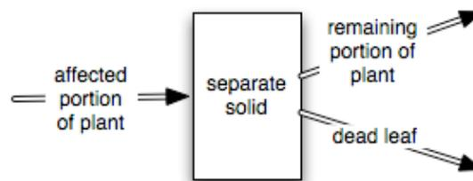
Figure 2. Functional modeling of plant sacrificing leaf
