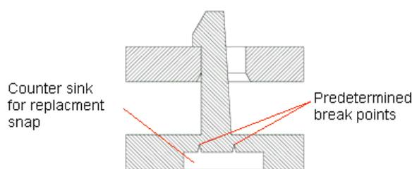
Figure 1a. Snap fit redesigned with countersink and break points
