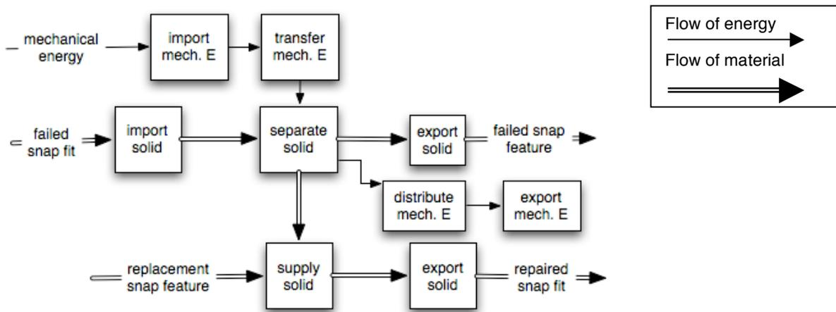
Figure 3. Functional model of repairing failed snap
