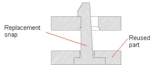
Figure 1b. Redesigned snap fit after failure and refurbishment
