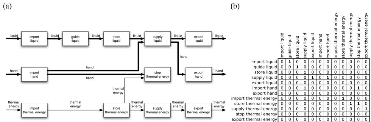
Figure 1. (a) A simple functional model and (b) the associated function-adjacency matrix.
