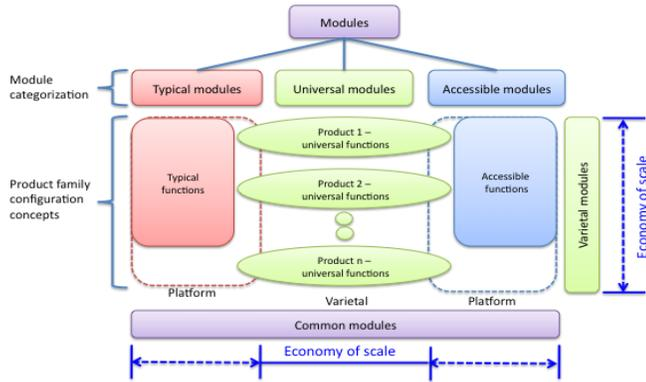
**Figure 2: Module categorization and platform based product configuration concepts**
